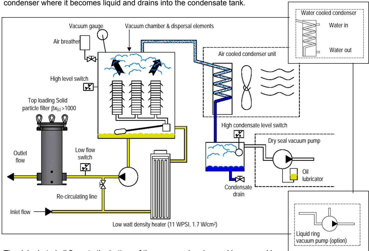
The dehydrated oil flows to the bottom of the vacuum chamber and is removed by the discharge pump. The oil is pumped through the high efficiency particulate filter assembly ( $\beta_{x[cl]} > 1000$ ) and returned to the system. The re-circulating line helps the VAC-U-DRY reach optimum temperature in cold start situations and can be used to throttle machine inlet and outlet flow.
